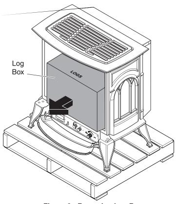
Figure 9 - Removing Log Box
